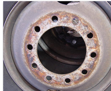
Steel Wheel performance after 3 years of service without using an Accuride Wheel-Guard
