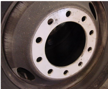
Steel Wheel performance after 3 years of service using an Accuride Wheel-Guard
