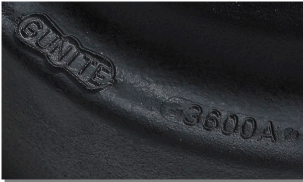
Close up of part number and Gunite logo in Gunite brake drum casting.
