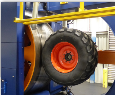
Radial Fatigue Test Machine for Large OHW Wheels
