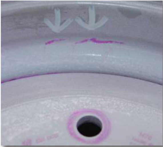
Crack in hump
