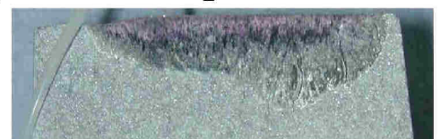
Fracture location in bolting area of an aluminum truck wheel (Hub B)
