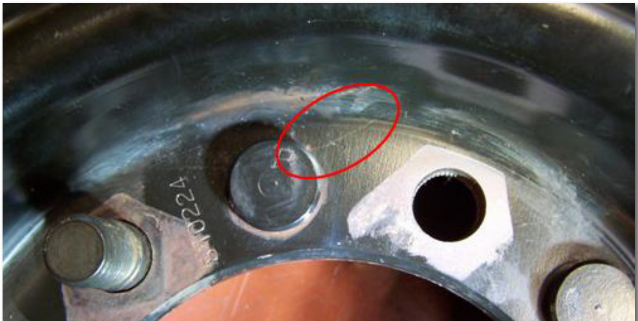
Crack out of an attachment hole
