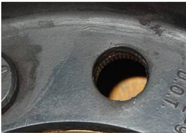
Stud got out of its place
