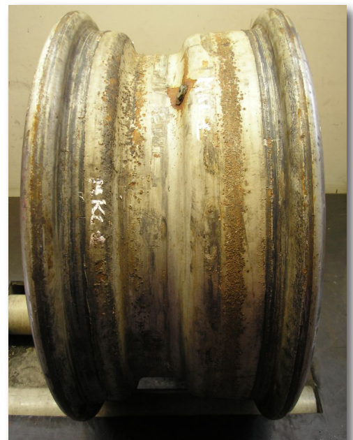
Dust and rust on the tyre sealing contact area
