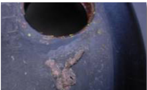
Amount of dirt in the sealing area
