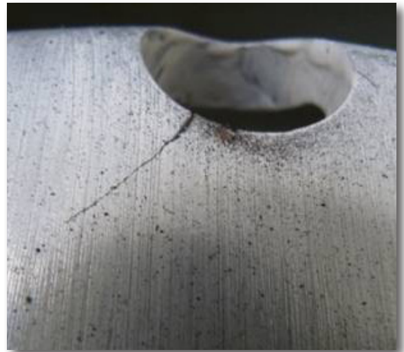
Crack at ventilation hole
