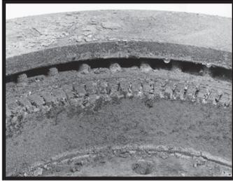
1. Un-treated cast iron where corrosion has destroyed the exciter teeth. Rotor must be replaced immediately.
