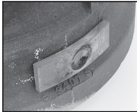
Welded balance weight
