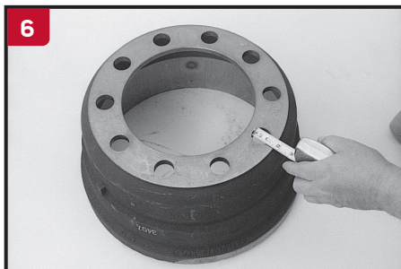
Number, size, and location of bolt holes
