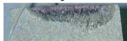
Fracture location in bolting area of an aluminum truck wheel (Hub B)
