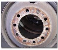
Steel Wheel performance after 3 years of service without using an Accuride Wheel-Guard
