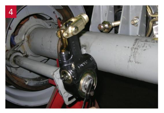
Install the slack onto the camshaft using the proper mounting hardware.
