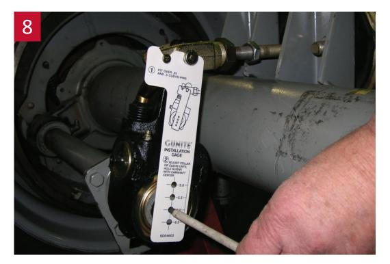
Align the slack by adjusting the  $\frac{34}{2}$  hex nut on the push rod until the appropriate centering hole on the template aligns with the center hole on the camshaft. The template is provided with centering holes for  $5^{\prime\prime}$ , 5.5<sup>"</sup>, 6<sup>"</sup>, and 6.5<sup>"</sup> slacks.
