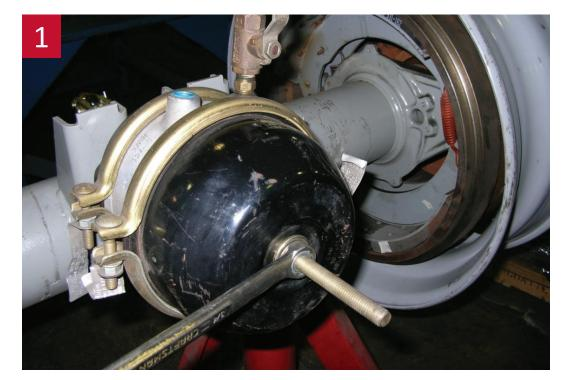
If the axle is equipped with spring brakes, manually cage the brakes following the manufacturer's recommended procedures.
