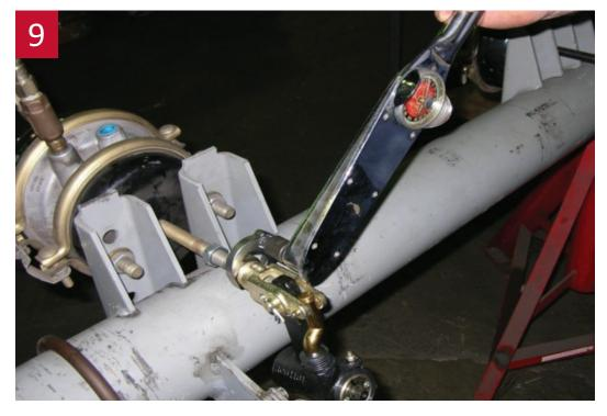
Using a torque wrench, tighten the 1-1/4" collar nut to the clevis using 40 - 50 ft. lbs. of torque.
