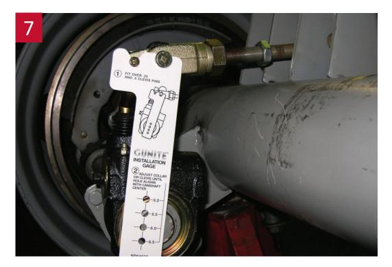
After threading the collar nut onto the clevis, place the template over the large and small clevis pins as shown above.
