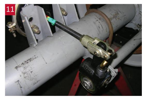
Fully apply the brakes and allow the chamber push rod to travel its maximum stroke. Clearance must exist between the slack adjuster and all adjacent chassis components. Release the brakes.
