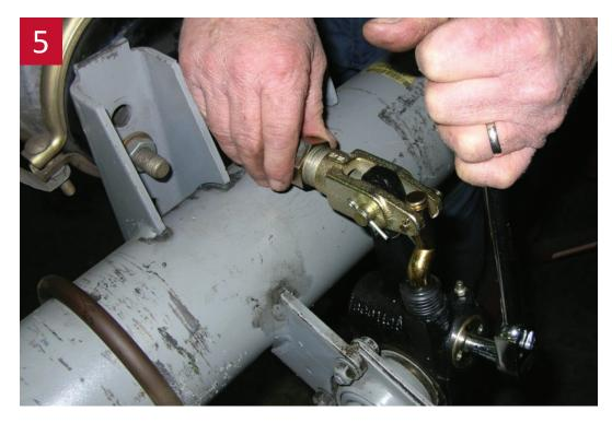
Using the hex extension and a wrench, adjust the slack so that the collar lock and nut aligns with the threaded area of the clevis.
