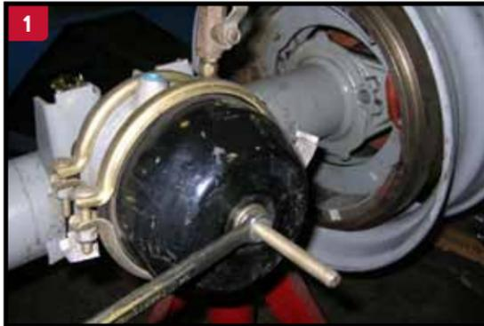
1 If the axle is equipped with spring brakes, manually cage the brakes following the manufacturer's recommended procedures.
