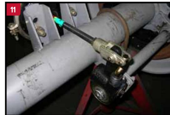
11 Fully apply the brakes and allow the chamber push rod to travel its maximum stroke. Clearance must exist between the slack adjuster and all adjacent chassis components. Release the brakes.
