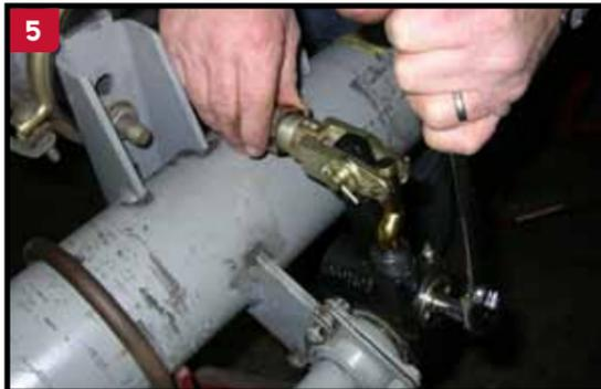
5 Using the hex extension and a wrench, adjust the slack so that the collar lock and nut aligns with the threaded area of the clevis.
