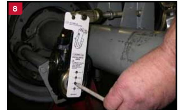
8 Align the slack by adjusting the 3/4" hex nut on the push rod until the appropriate centering hole on the template aligns with the center hole on the camshaft. The template is provided with centering holes for 5", 5.5", 6", 6.5" slacks.
