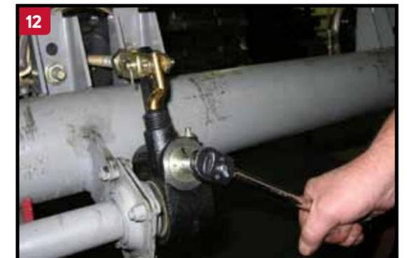
12 Pre-adjust the brakes by rotating the hex extension clockwise until the brake lining contacts the brake drum. Back the slack adjuster off by rotating the hex counterclockwise 1/2 turn. Backing off a new slack adjuster will require up to 50 ft. lbs. of torque. A ratcheting sound will be heard when backing the slack off. After completing this step, uncage the spring brake.
