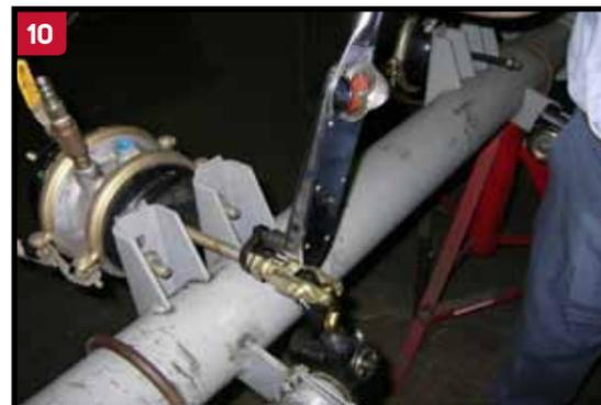
10 Once the 1-1/4" collar nut has been properly tightened to the clevis, tighten the 15/16" jam nut against the collar lock nut using 40 to 50 ft. lbs. of torque.
