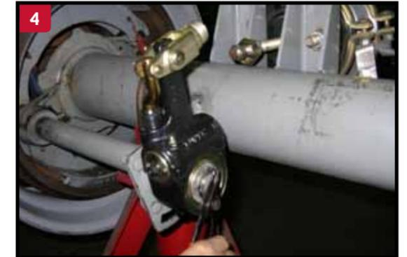
4 Install the slack adjuster onto the camshaft using at least one inner washer to align the slack adjuster with the brake chamber push rod and enough outer washers to allow no more than 0.060" movement of the slack adjuster on the camshaft. Secure with the snap ring.
