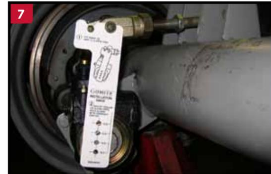
7 After threading the collar nut onto the clevis, place the template over the large and small clevis pins as shown above.
