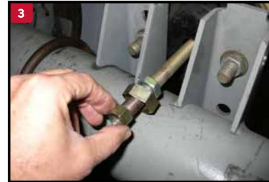
3 When installing a Gunite slack adjuster with a collar lock clevis, place the 1-1/4" collar nut on the push rod against the 15/16" jam nut. Next thread the 3/4" hex nut onto the push rod.
