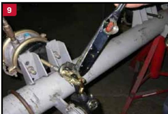
9 Using a torque wrench, tighten the 1-1/4" collar nut to the clevis using 40 to 50 ft. lbs. of torque.
