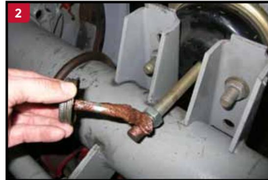
2 Apply anti-seize to the chamber push rod threads before installing the new clevis. Also apply anti-seize to the camshaft splines at this time.
