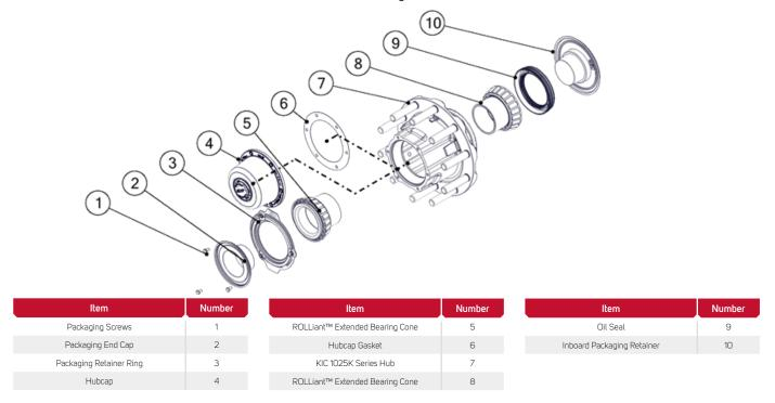
Figure 1. ROLLiant™ components. SAE P spindle hub shown, other configurations are similar.
