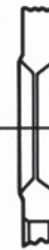
Chamfer extruded on side opposite nut. Causes: Too much torque or improper nut.
