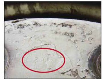
Visible signs that paint exceeds the maximum allowable thickness of 3.5 mils. Multiple coats, uneven surfaces, and illegible stampings indicate too much paint.
