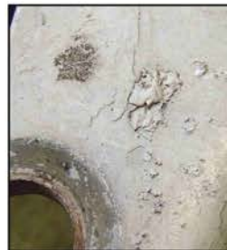
Visible signs that paint exceeds the maximum allowable thickness of 3.5 mils. Multiple coats, uneven surfaces, and illegible stampings indicate too much paint.
