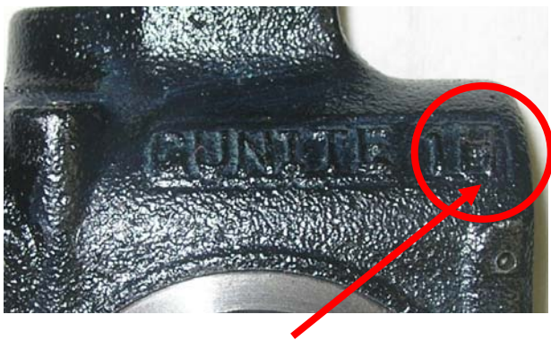
Figure A: Mold Line Nomenclature
