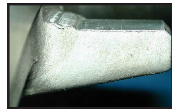
Damage to aluminum hub pilots will not allow the drum to seat properly.
