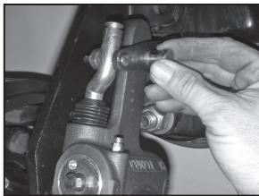
**3.** Insert the large and small pins in the proper clevis holes.
