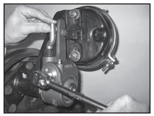
2. Using a 7/16" wrench or a socket, rotate the hex extension clockwise until the holes in the Gunite automatic slack adjuster are properly aligned with the corresponding holes in the welded clevis. Hold the link down while rotating the hex extension clockwise. Failure to do so can cause the link to disengage from the drive. Do not use an air impact wrench on the 7/16" hex. It can damage the clutch.
