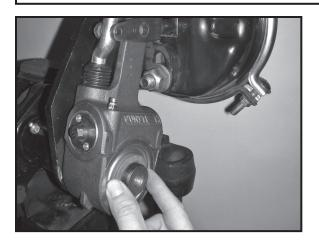
Apply anti-seize compound to the camshaft and install the automatic slack adjuster using the original mounting hardware. Properly shim the automatic slack adjuster using the existing washers onto the camshaft to ensure alignment with the brake chamber's push rod. Re-attach the retaining clip.
