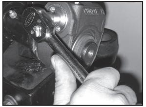
5. Uncage the spring brake then fully apply the brakes and allow the chamber push rod to travel its maximum stroke. Clearance must exist between the Gunite automatic slack adjuster and all adjacent chassis components. Release the brakes. After completing this step, refer to section on Brake Adjustment After Installation.
